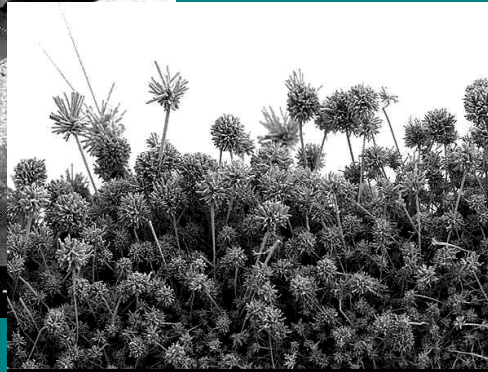
Chemical vapor deposited copper oxide---5kV---100X courtesy of Jim Steitz, Air Products Co.
