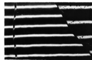
Figure 3. Microinterferogram showing multiple-beam Fizeau fringes crossing a Cashmeline fibre immersed in a liquid with refractive index n_2 = 1.5240 .
