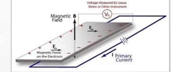
• WHEN A CURRENT-CARRYING CONDUCTOR IS PLACED INTO A MAGNETIC FIELD, A VOLTAGE WILL BE GENERATED PERPENDICULAR TO BOTH THE CURRENT AND THE FIELD.
