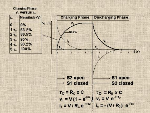
The Voltage V<sub>c</sub> and the current i<sub>c</sub> during the charging phase and Discharging phase.
