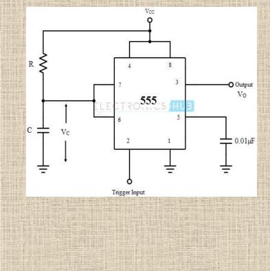
R is connected between pin 4,pin 8 and pin 7, pin 6. The capacitor C is connected between pin 6 and pin 7 and ground . Trigger input pulse of voltage is given externally to pin 2. pin 1 and pin 5 is ,capacitor is grounded. Pin 4 and 8 are connected to +Vcc which can be between 5 v to 15 v.
