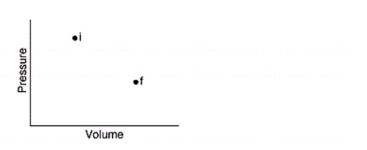
A p-V diagram showing the initial state i and the final state f of the free expansion
