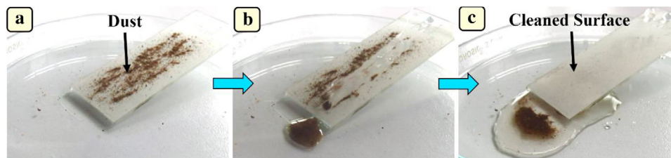
Figure 5. A self-cleaning behavior of P-2 sample.
