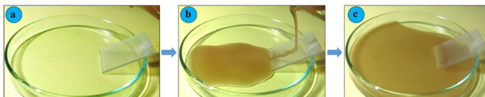
Figure 6. a-c) Self-cleaning behavior of superhydrophobic coating.
