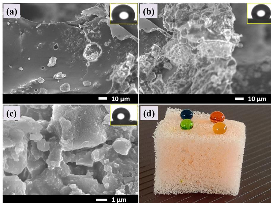
**Figure 1.** Scanning electron microscopy images of a) S1, b) S2 and c) S3 samples. d) The optical photograph of color water drops placed on S3 sample.
