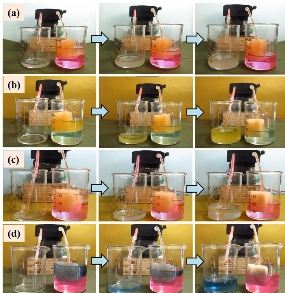
**Figure 2.** Continuous oil collection using a peristaltic pump a) diesel, b) petrol, c) coconut, and d) kerosene from oil–water mixture.
