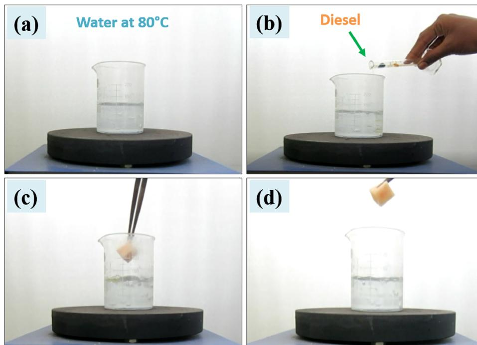
**Figure 4.** The oil–water separation by S3 sample from oil–hot water mixture.
