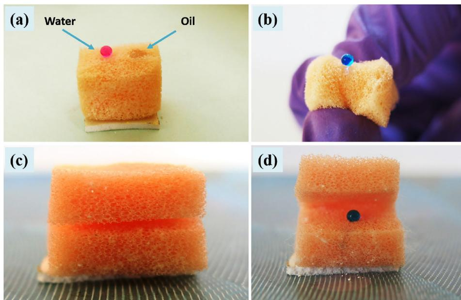
**Figure 3.** a) Optical image of water and oil drop on S3 sample, b) twisting of S3 sample and c–d) S3 sample cut in middle part and checked its wettability.
