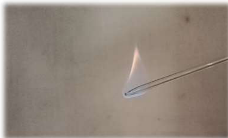
Figure 7 Flaming test for Bio Methane
