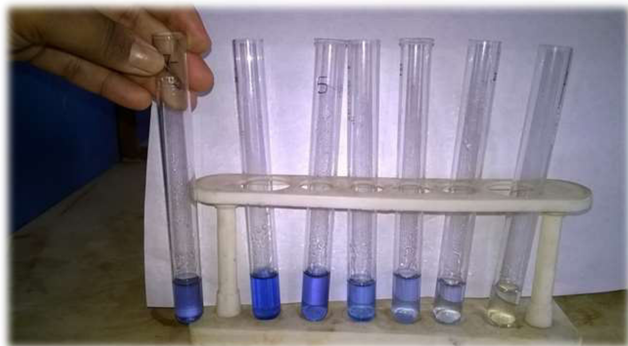
Figure 9: Estimation of Deoxyribose Sugar by Diphenylamine Method
