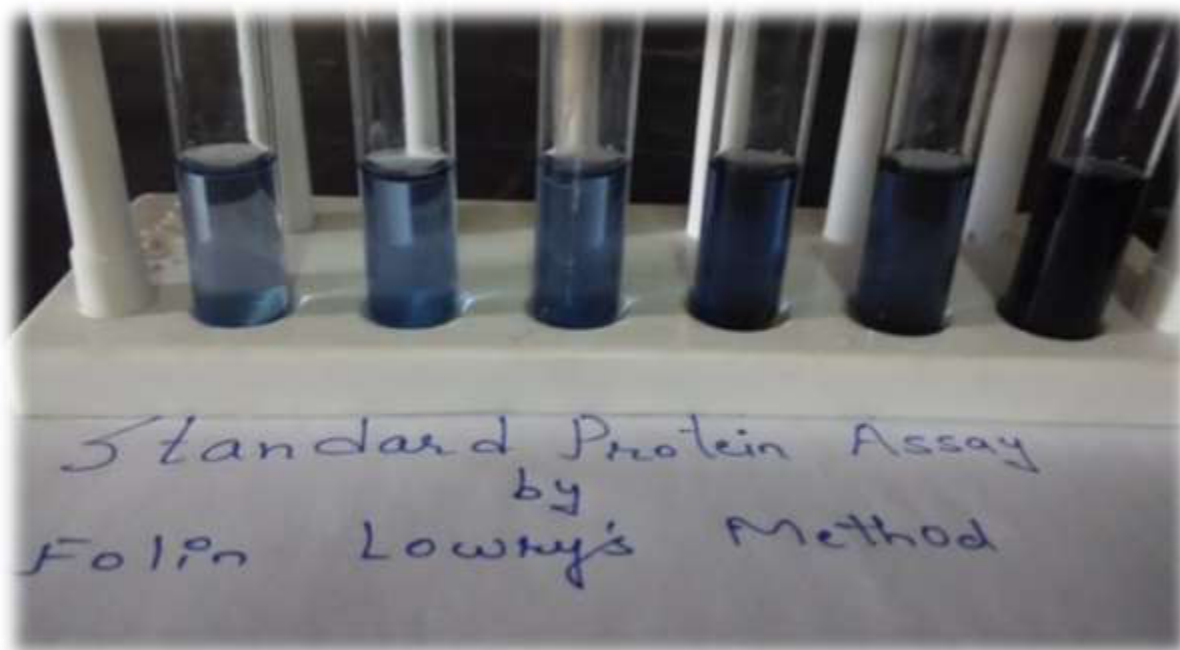
Figure 12 Estimation of Protein by Lowry's Method
