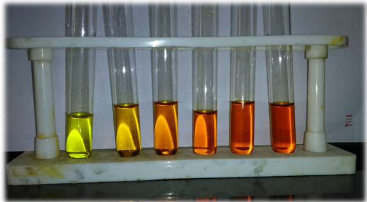
Figure 10: Estimation of Reducing Sugar by DNSA Method
