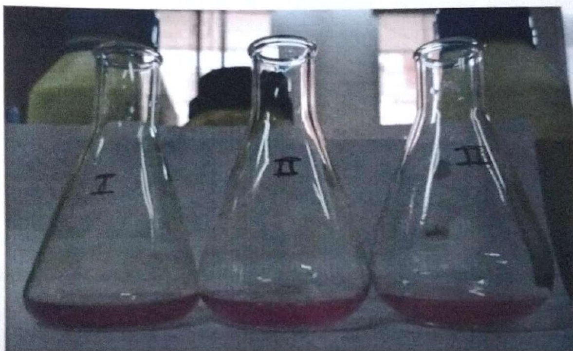
Fig. 6). Result of titration by 2, 6 dichlorophenol indophenol method (colourless to light pink)
