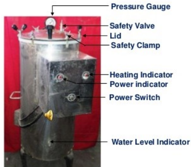
Figure. Autoclave unit used for wet sterilization of nutrient media
