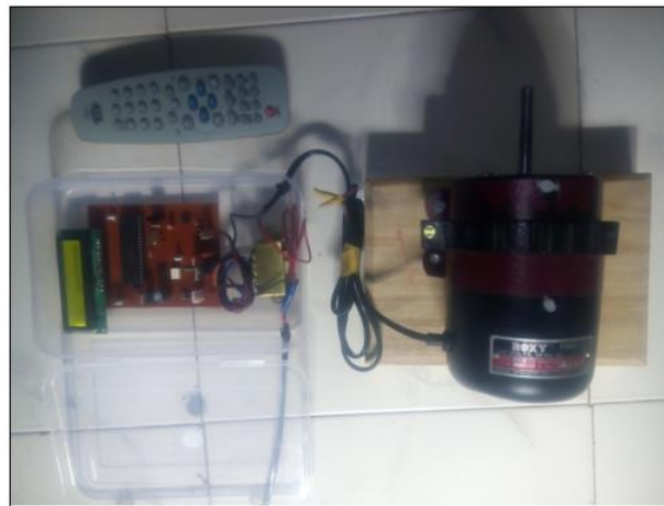
Fig.5. Hardware of the IR TV remote based speed control of single phase AC motor
