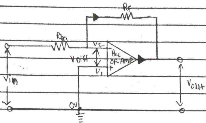
In this inverting Amplifier circuit the operational amplifier is connected with feedback of produce when the dealing operational amplifier there are two very important rules remember about inverting amplifier these are
