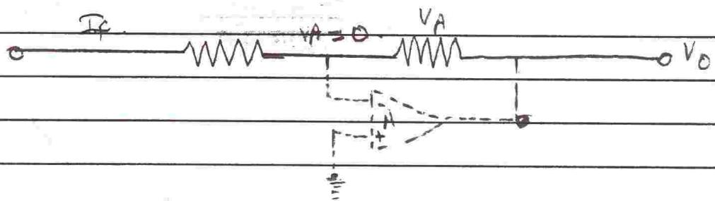
This because junction is input and feedback signal ( $\times$ ) of some potential of positive (+) input which is zero volt and ground then the junction is virtual ground.
