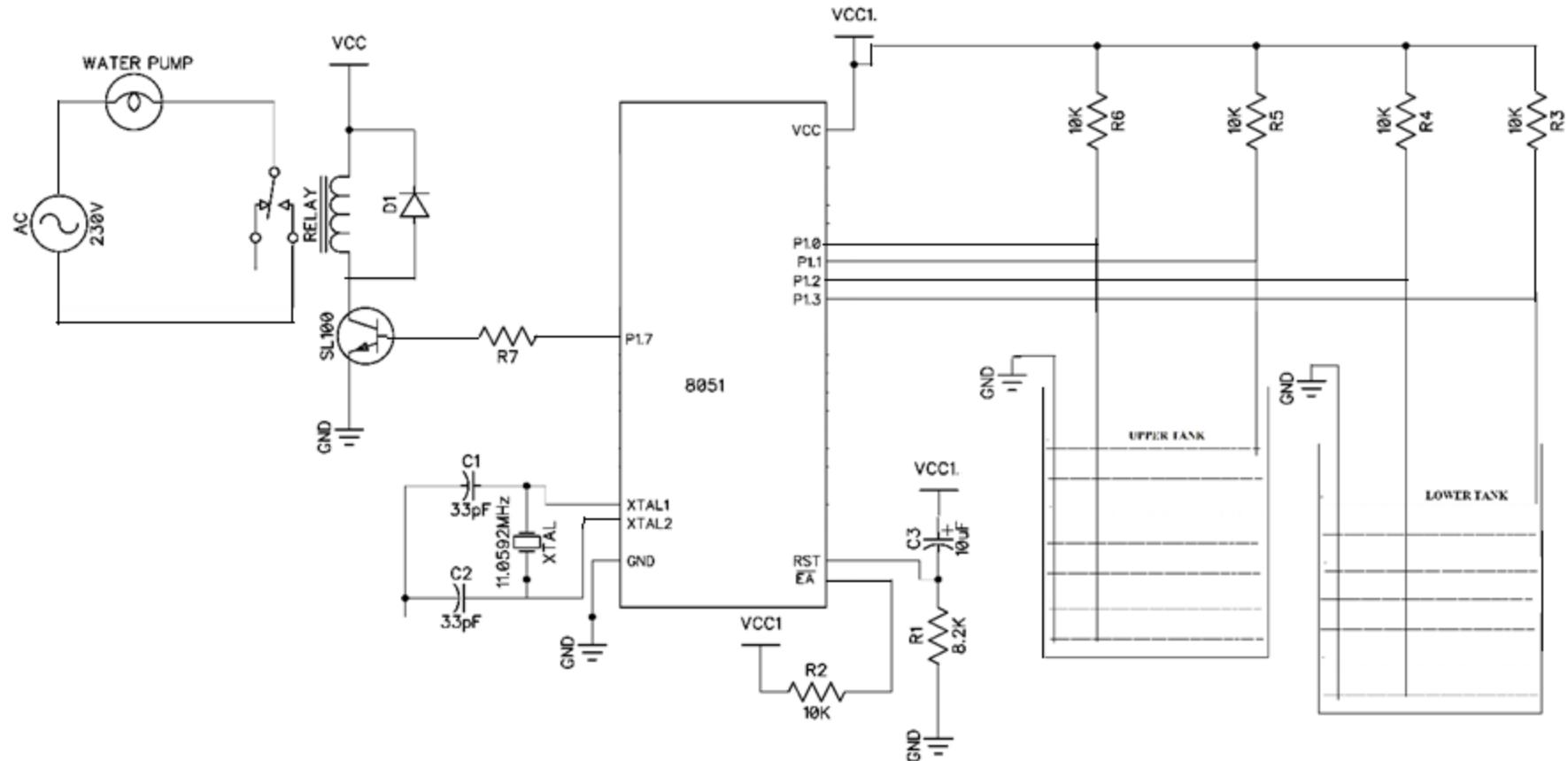
The complete circuit schematic of the water level controller using 8051 is as shown in fig 4.5. Here port P1 pins P1.0, P1.1 ,P1.2 and P1.3 are used to monitor the statues of the tanks. Here the system is developed by considering two tanks upper and lower.
