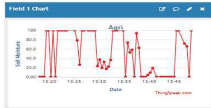
Figure 1.7 (a): Soil moisture data on ThingSpeak platform
