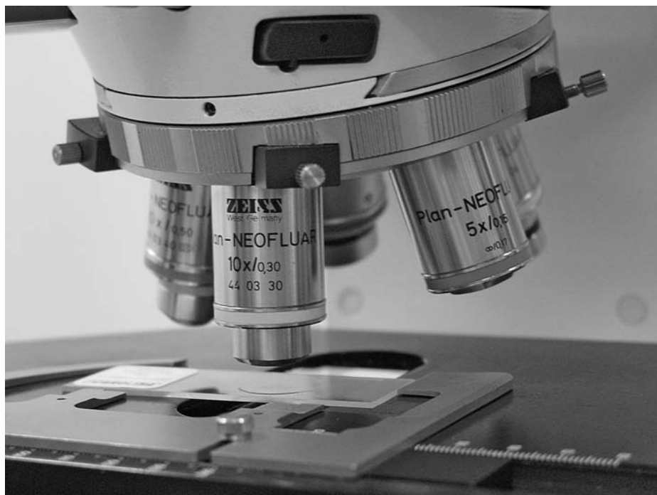
Fig. 4.4 The objective lens. A selection of objective lenses mounted on an upright research grade compound light microscope. From the inscription on the two lenses in focus they are relatively low magnification 10\times and 5\times of numerical aperture (NA) 0.3 and 0.16 respectively. Both lenses are Plan Neofluar, which means they are relatively well corrected. The 10\times lens is directly above a specimen mounted on a slide and coverslip, and held in place on the specimen stage.
