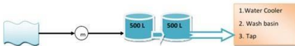
Figure No.5.3 Schematic diagram of Water Source, Storage and Usage for Municipal water Supply
